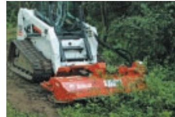
Flail Cutter clears brush and small trees up to 3-in. in diameter.
