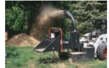
Chipper grinds branches and reduces volume 10-to-1.
