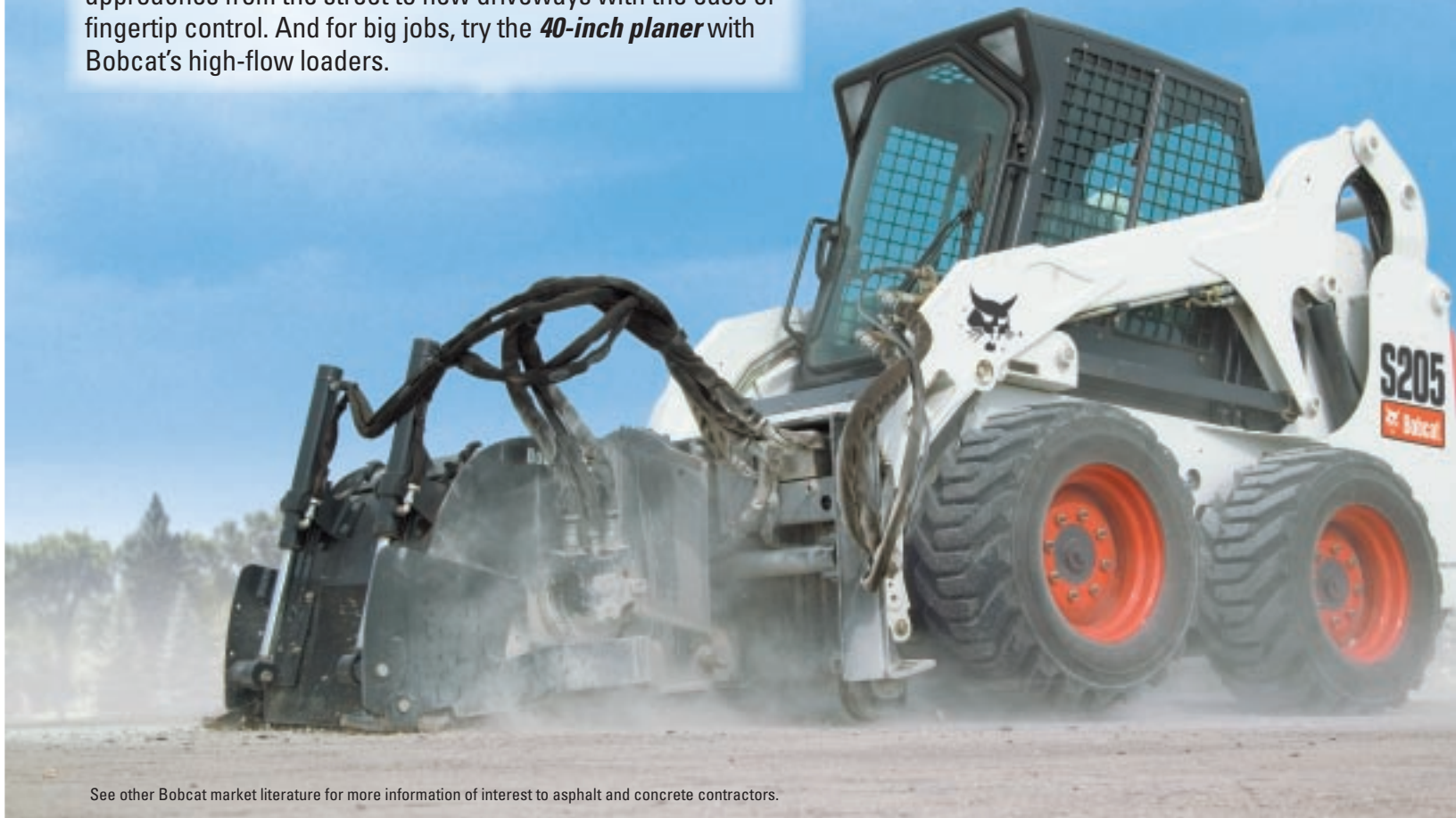
Curb Planer mills concrete curbs to create smooth approach from driveway to street.
