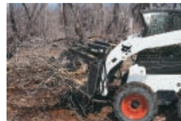
Industrial Grapple easily clamps, sorts and removes debris.
